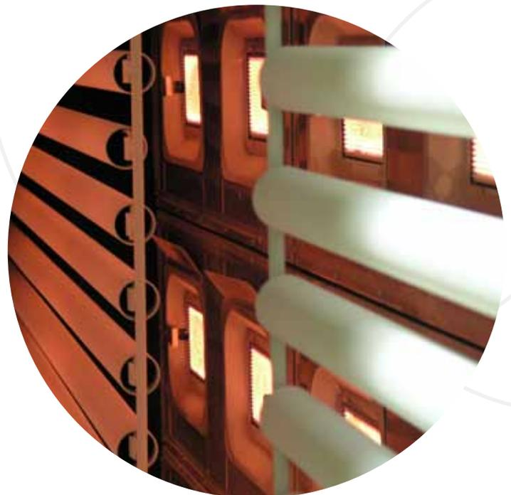
Hard anodising produces thick, abrasion resistant films. Using a low temperature electrolyte, films of up to 125 microns can be produced.
